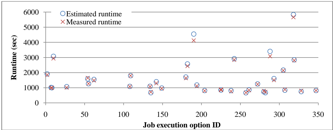
Figure 55. Experimental runtime data for real-world resources for selected job execution options. Circles represent job execution option runtime estimation generated by OptionView while x’s represent observed runtime characteristics after job’s execution on real-world resources as per instructions of the job plan generated by OptionView.
