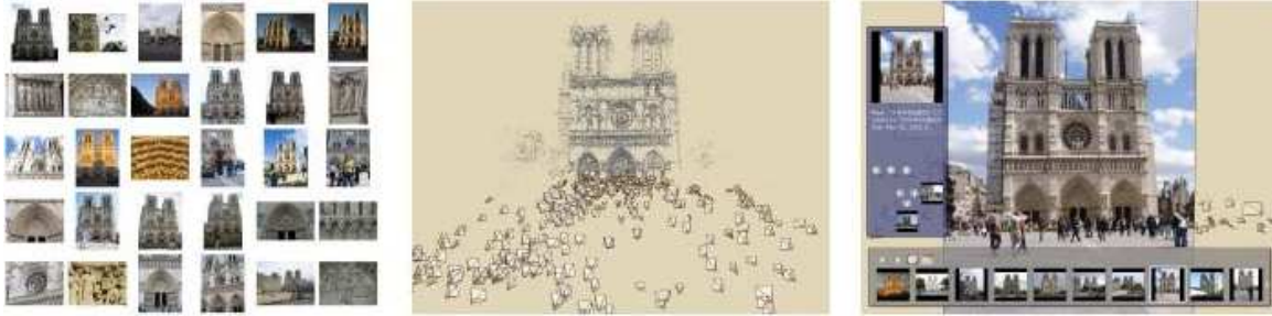
Figure 2.4: An illustration of the system of Photo Tourism. Offline, the system takes as input an image collection of a tourist attraction (left) and automatically reconstructs a sparse set of 3D points and the camera parameters (center). During online exploration, Photo Tourism renders both the enhanced scene points as well as the camera viewpoints in 3D, and allows the user to select different viewpoints and browse the corresponding images (right). This figure is cited from [95].
