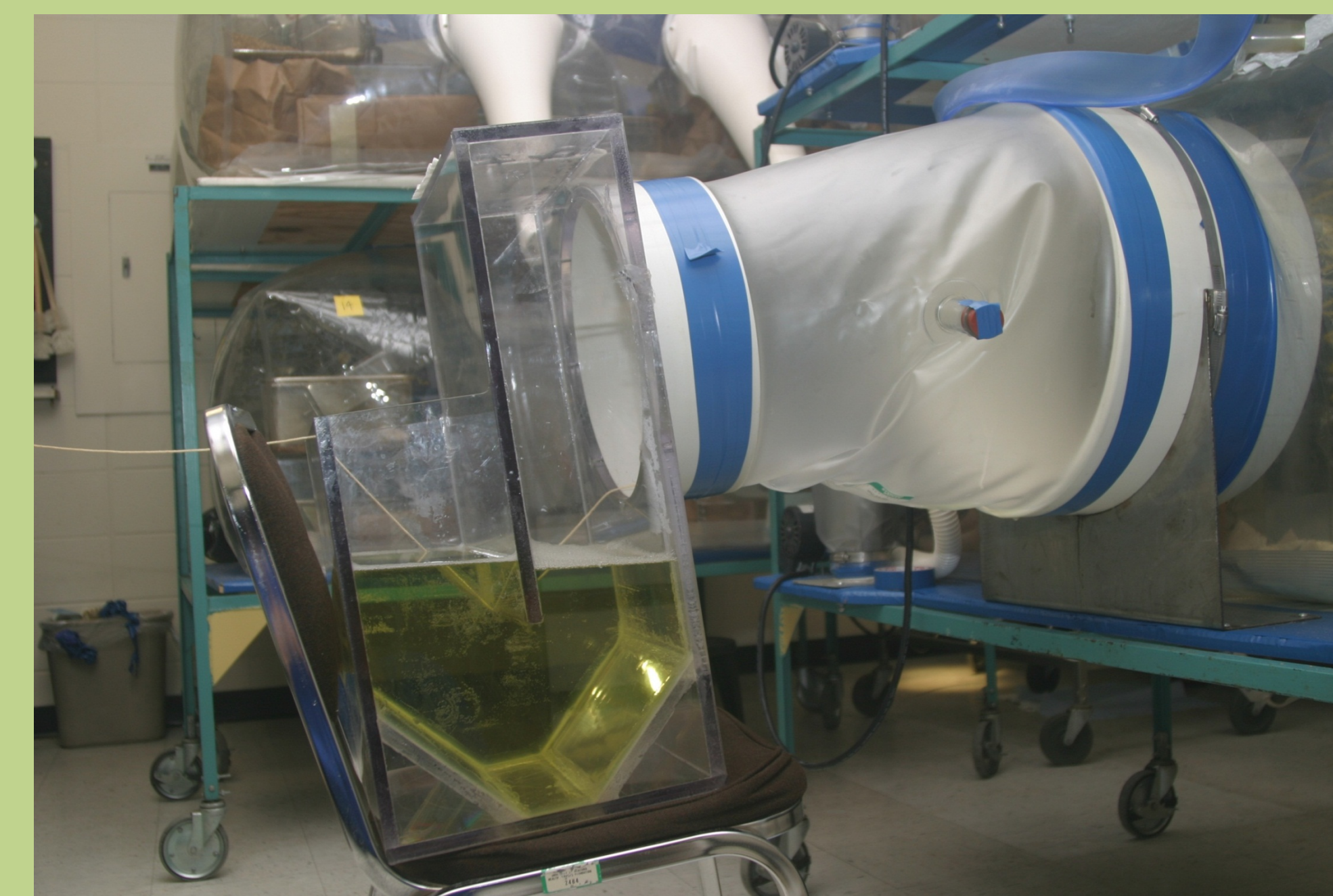
Sterilant-filled trap connected to isolator
