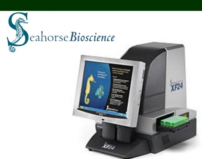
The XF24 Analyzer measures oxygen consumption rate (OCR) and extracellular acidification rate (ECAR) at intervals of approximately 2-5 minutes. OCR is an indicator of mitochondrial respiration, and ECAR is predominately the result of glycolysis.
